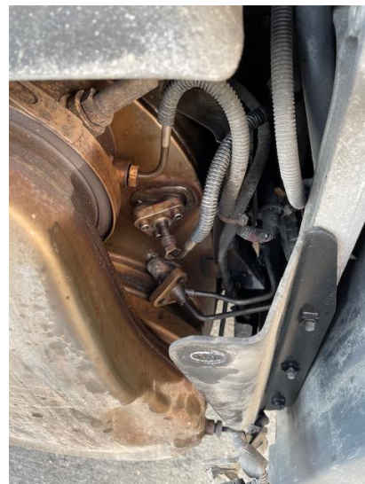
Figure 2. Montage assembly sensor on catalyst
